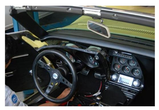
A top priority was to get the odometer repaired, so I would be able to track the fuel economy. Some "while your at it" reasoning resulted in having the tachometer, which is like the speedometer in that both are mechanical, rebuilt. The light switch was also replaced because the instrument panel dimmer was not working properly.
