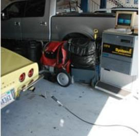
The idle setting is adjusted with the aid of a "Emissions Inspection Analyzer". There's a bit of irony here - a '68 Corvette hooked up to a smog machine. It's about the only time that will happen as '68s are exempt from any smog inspection requirements here in California - one of the few breaks we get with these cars.
