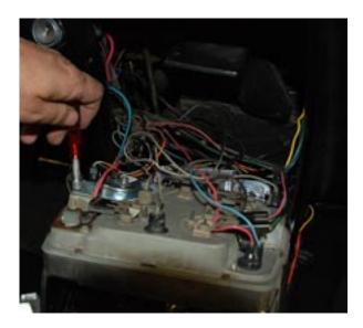
Replacing the clock went as well as could be reasonably expected. Once access to the gauge console is obtained it's a simple matter of removing two bolts with a nut driver, disconnecting the one electrical terminal for the clock and removing the bulb / socket and installing the new clock as illustrated above. I then proceeded to open a brew and congratulate myself on a job well done.\
