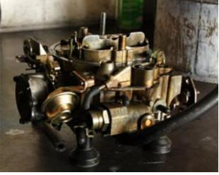
Introducing the Rochester Quadrajet Carburetor. It made it's first appearance in the Corvette in 1968; previously Holley products had been used. The Holley and
